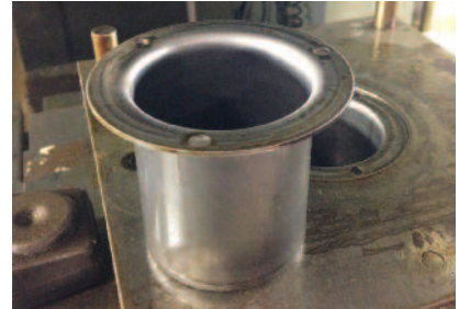
TOP: Tonnard formed this muffler tip from 0.036 in. cold-rolled steel for a 1930s antique motorcycle.
