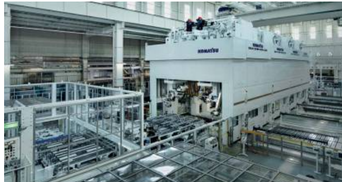
Large-sized Servo Press line for stamping automotive body panels
